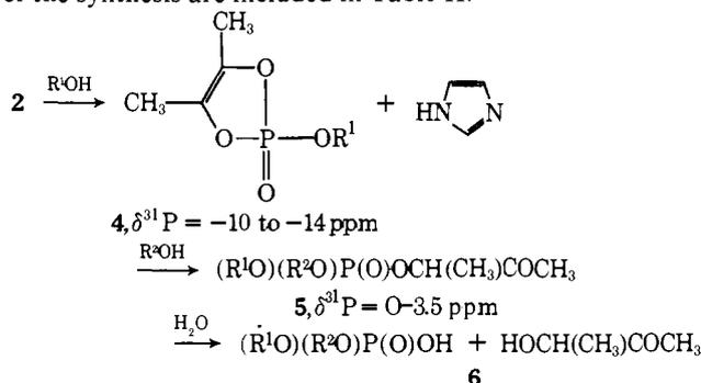
The phosphorylimidazole **2** need not be isolated in the phosphotriester synthesis because it is generated rapidly and quantitatively from imidazole and the pyrophosphate **1** in dichloromethane solution, and because the salt **3**, which is formed as by-product, does not react with alcohols at appreciable rates.<sup>20</sup> The salt **3** is readily separated from the triester **5** in the work-up. Several applications of this procedure 2B are listed in Table II.
